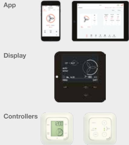
Anything is possible – from a simple display on the unit, to a practical app that can be used on the go, right through to fully automated, demand-based ventilation using sensors. You can also integrate Zehnder ComfoAir Q into a building control system via the KNX interface.
